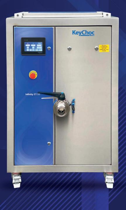
Seed tempering as in a traditional wheel machine, but with a much more stable temper and all the functionality of the latest continuous tempering machines.
